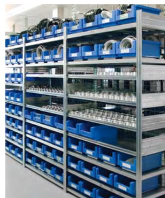
The e-nventory rack systems are only 400 mm deep and contain two to three times more articles than a two-bin Kanban system in the same space.
