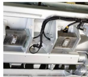
*4-wire connection: Pluggable, easy to lay, inexpensive: the new 4-wire cells*
