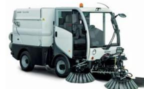
DIGI SENS sensors indicate to the driver when the refuse container reaches the weight limit.
