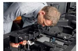
Mounting a sensor on to a lorry chassis for tests.
