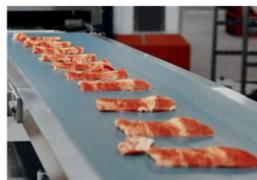
Measurement on the moving conveyor belt – DIGI SENS sensors monitor the weight of every portion.
