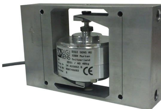
systems to be built using one load cell (monobloc construction), where normally three or more conventional cells would be required.
